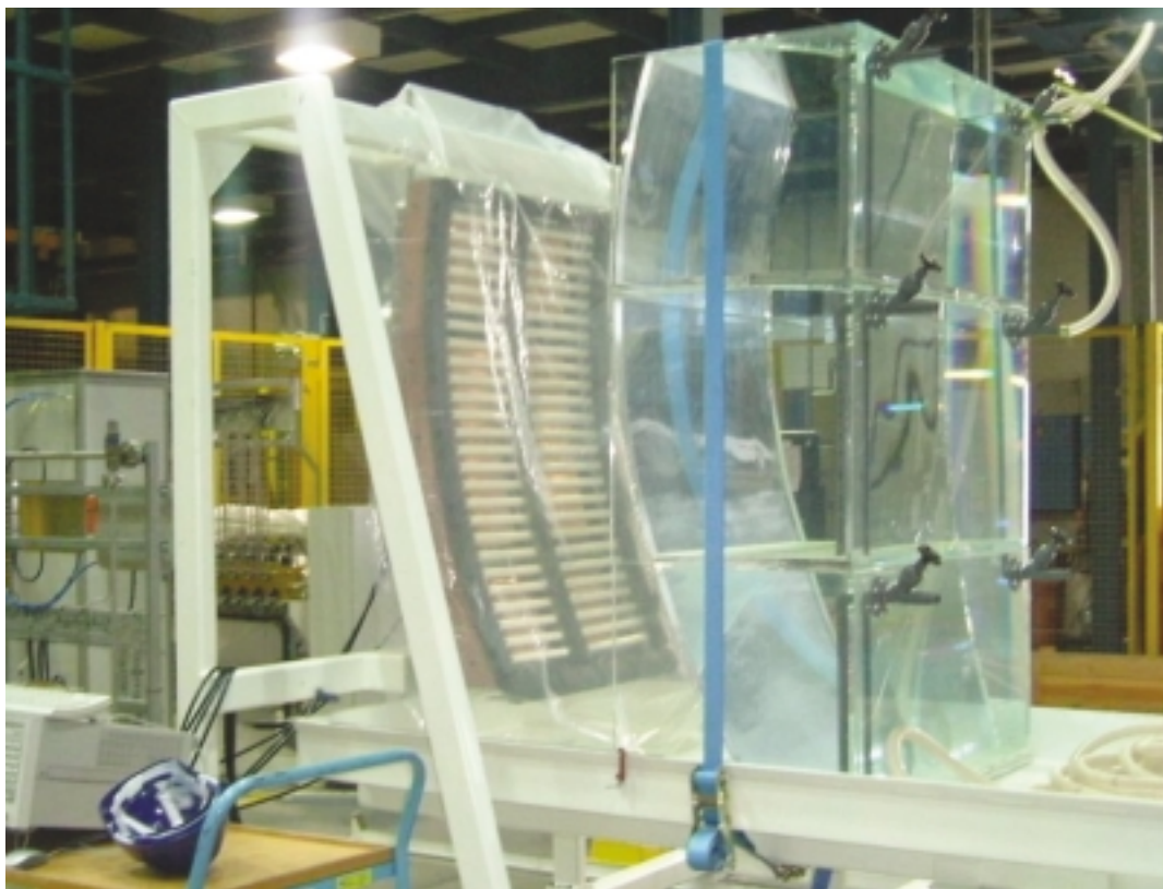
Figure1: View of ILA antenna housing and the salted waterload during the measurements of the ILA impedance matrix
