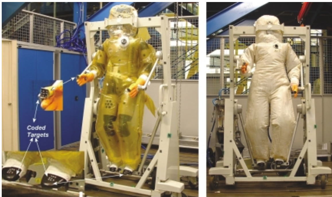
Figure 1: Left: Coded targets on frame and limb extremes active macro producing CAD mannequin position. Right: Suit painted for surface measurement.
