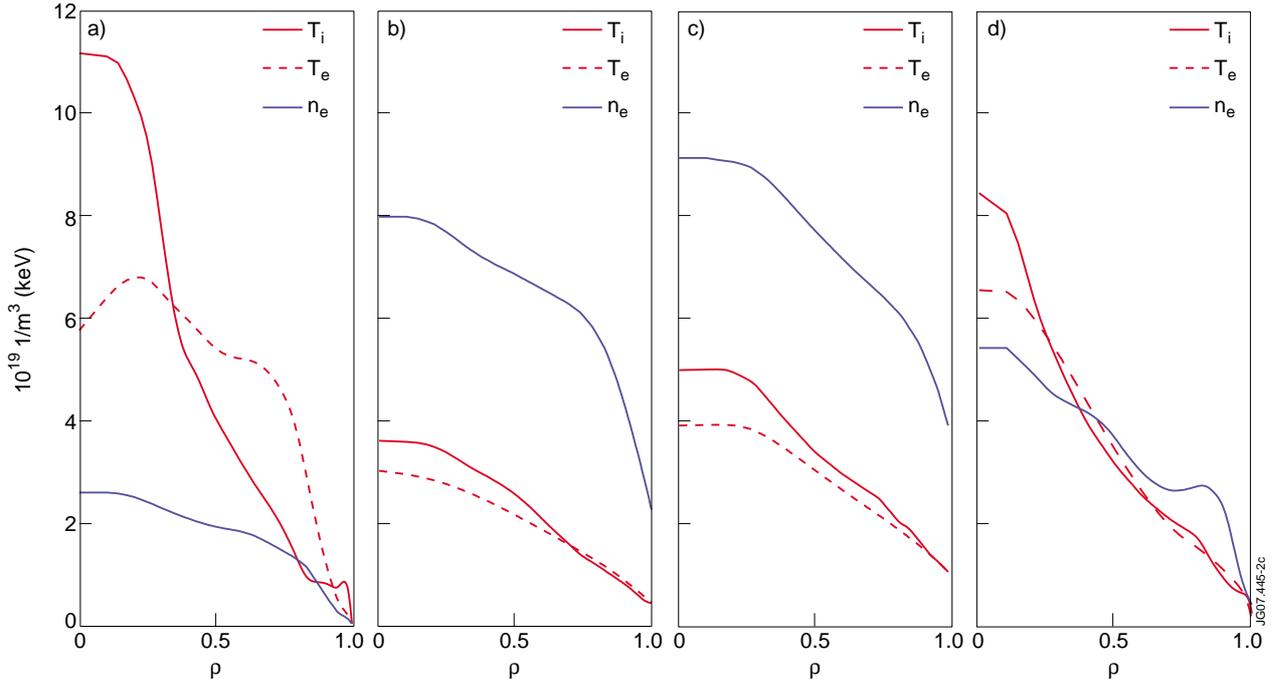
Figure 1: Temperature and density as functions of the normalized poloidal flux  $\rho$  for the discharges a) Pulse No's: 51976 at  $t = 4.8s$ , b) 50844 at  $t = 21.5s$ , c) 52009 at  $t = 21.0s$ , and d) 66498 at  $t = 7.1s$ . The ion temperature profiles indicate that a) and d) are advanced scenario discharges with an ITB, whereas b) and c) are ELMy H-mode discharges.
