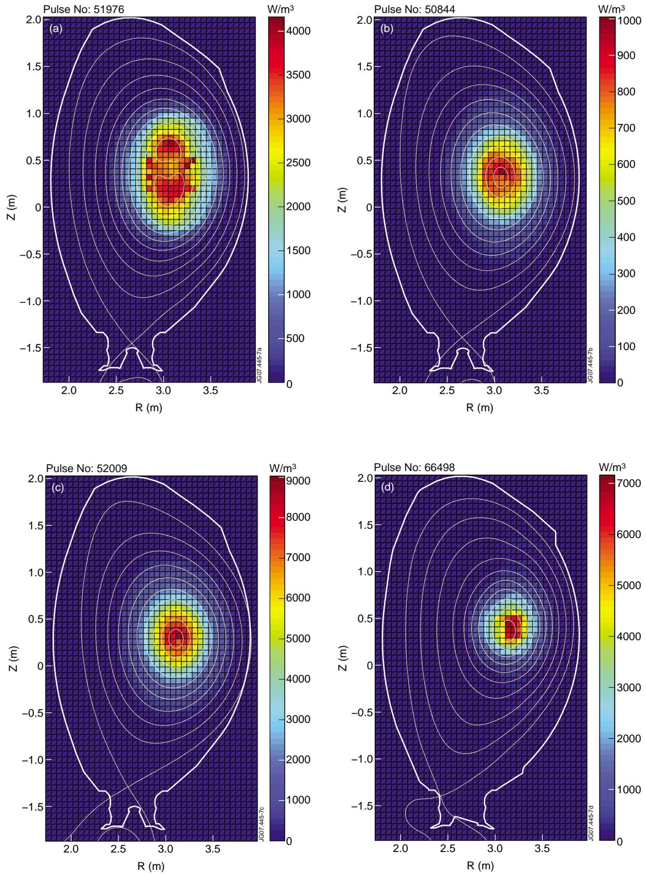
Figure 3: The alpha power deposition profiles in Pulse No's: a) 51976, b) 50844, c) 52009, and d) 66498.
