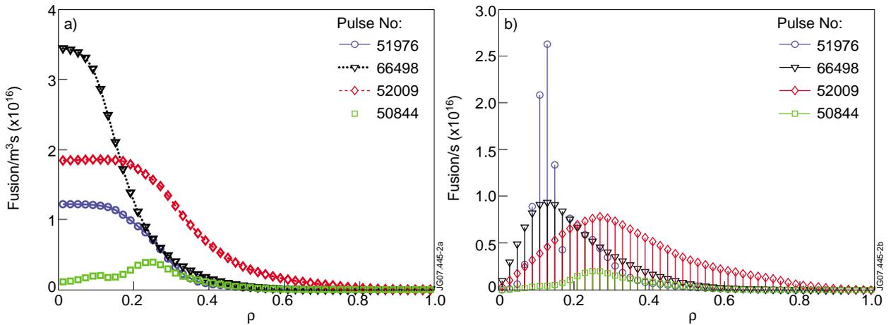
Figure 2: a) fusion reactivities and b) fusion reaction rates of the studied discharges. Total power to alpha particles, obtained summing up the fusion rates in b), and multiplying them by  $3.5MeV$  were:  $69.5kW$  (Pulse No: 51976),  $13.6kW$  (Pulse No: 50844),  $87.8 kW$  (Pulse No: 52009), and  $42.1 kW$  (Pulse No: 66498).
