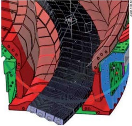
Figure 1: Location of the bulk tungsten row (LB-SRP) in the divertor of JET
