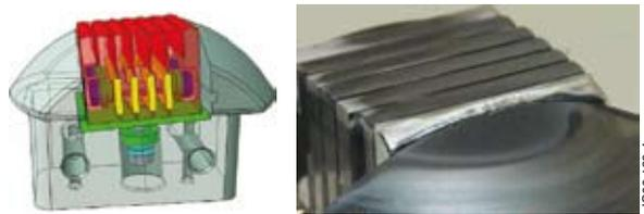
Figure 4: Partially molten mini-prototype after exposure to a TEXTOR plasma ( $E_{dep} > 130 \text{ MJ/m}^2$  on front side)
