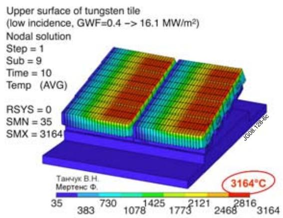
Figure 6: Temperatures reached on the upper surface of tungsten tiles in the case of low incidence, Global Wetted Fraction GWF=0.4,  $P_{dep} = 16.1 \text{ MW/m}^2$  for 10s
