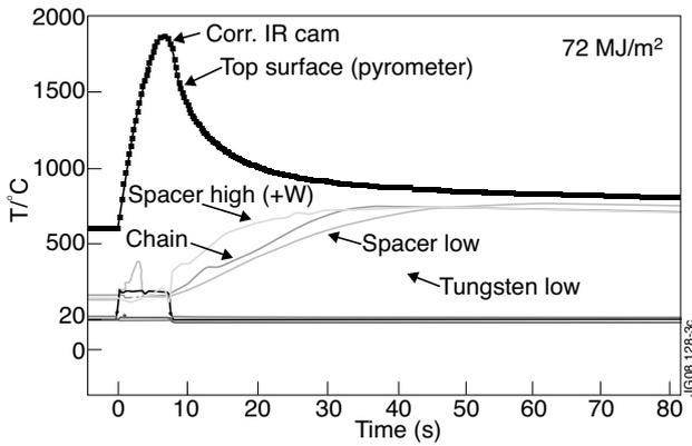
Figure 3: Temperatures recorded at different points in a prototype stack exposed to an electron beam flux of  $72 \text{ MJ/m}^2$  in the JUDITH-2 facility
