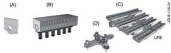
Figure 2: Components and assemblies of the bulk-W divertor unit
