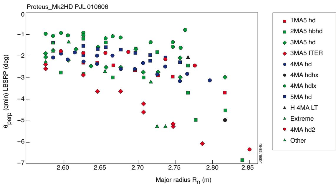
Figure 5: Angles of incidence of the magnetic field on the bulk tungsten tiles,  $\theta_{perp}$  versus major radius  $R_0$
