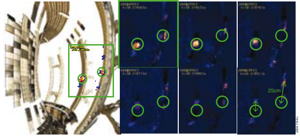
Figure 6: Evolution of filament impacts on the outer limiters. The poloidal drift of the strike point is attributed mainly to the toroidal rotation of the filament. The interframe separation is 71 \mu s (displaying one every two frames). The circles are fixed on the initial position of the interaction point.
