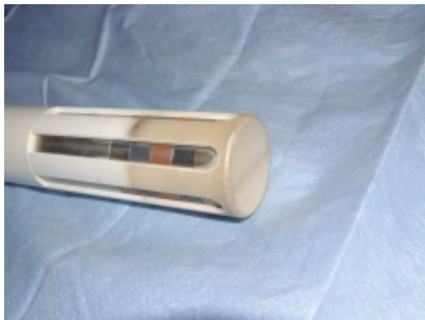
Figure 1: View of the activation probe after an irradiation by 63 JET plasmas
