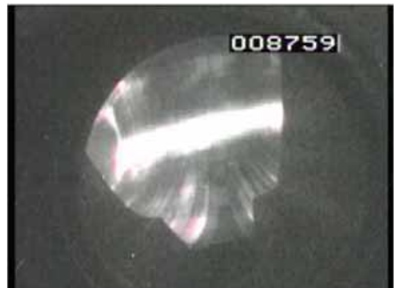
Figure4: Example of MARFE growing from FTU Pulse No: 22214
