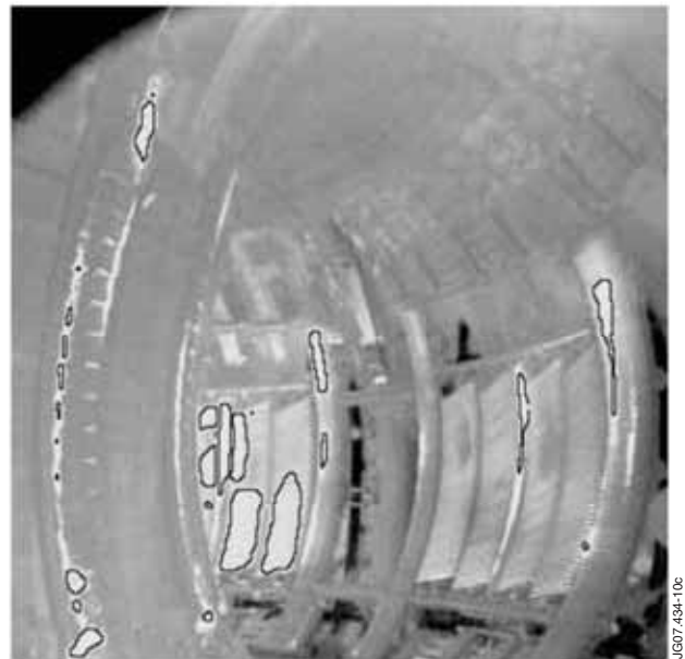
Figure 10: Example of static detection of hot spots. The contour of the detected regions is reported superimposed to the starting frame.
