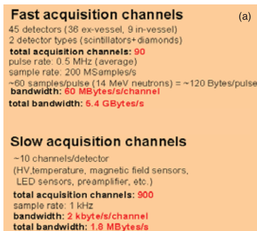
Figure 4: (a) RNC data acquisition requirements; (b) expected 14MeV n count rates with NE213 (1% efficiency) and diamonds (0.01% efficiency) for ITER scenario2 (MCNP calculations).
