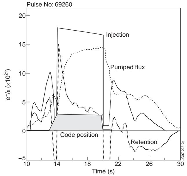
Figure 2: Particle fluxes for a typical pulse of the Type I ELMy H-mode series. The long term retention dominates the retention after 6 sec.
