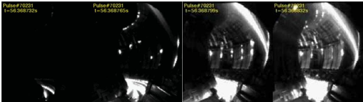
Figure 4. ELM onset and interaction with the wall (@ 30 kfps 25 \mu s exposure). A helical wall-interaction pattern can be seen less than 40 \mu s after the start of the D_{\alpha} rise.
