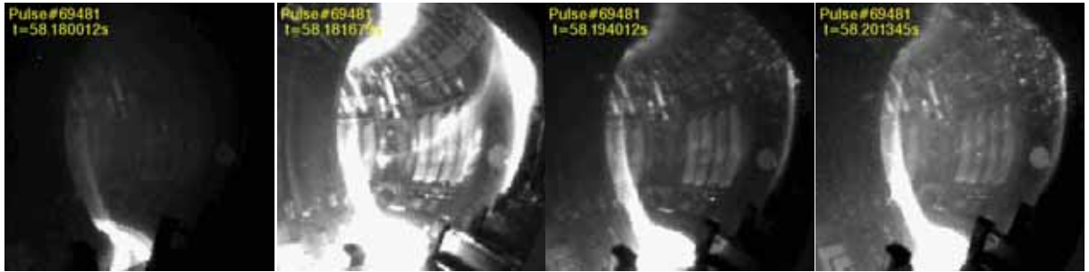
Figure 1. Particle expulsion from a poloidal limiter. Images are taken at 3 kfps with 166 \mu s exposure time.
