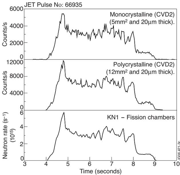
Figure 3: Comparison of time dependent neutron emission measured at JET by fission chambers, and two types of CVD diamond detectors: polycrystalline (CVD1) and monocrystalline (CVD2).
