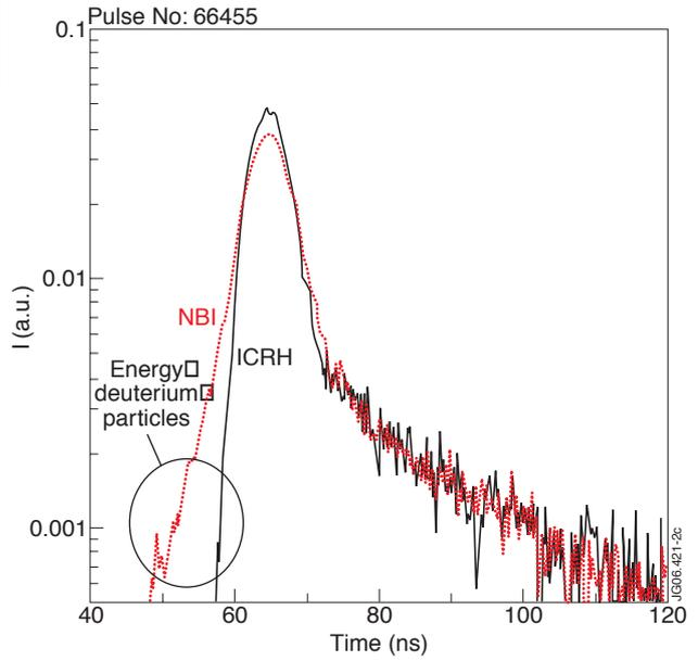
Figure 2: Neutron emission spectra measured with TOFOR from JET discharge #66455 during a phase with NBI (black) and during a phase with ICRH heating (red).
