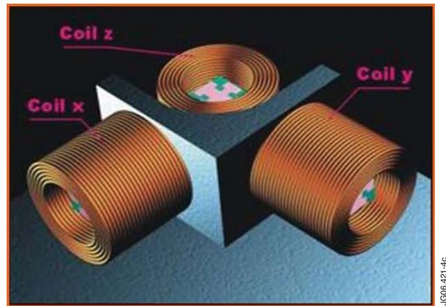
Figure 4: Overview of the three dimensional hard Hall probe assembly, showing the coils wound around the three Hall sensor.
