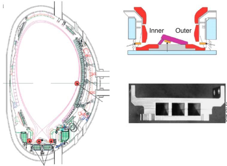
Figure 5: a),b) The locations of the mirror test units inside JET vacuum vessel, c) one of the cassette assembly containing the mirror materials.
