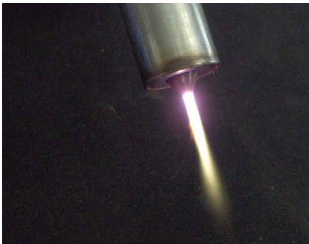
Figure 3: Image of the small size plasma torch working in nitrogen (300 W, 8000 sccm).
