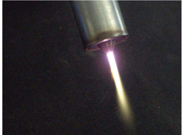
Figure 2: Picture of a Nitrogen plasma torch in operation. The plasma plume is 4cm long and the diameter of the torch itself is 2cm.
