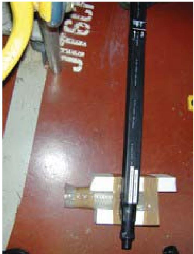
Figure 8: Collar probe as marked before installation
