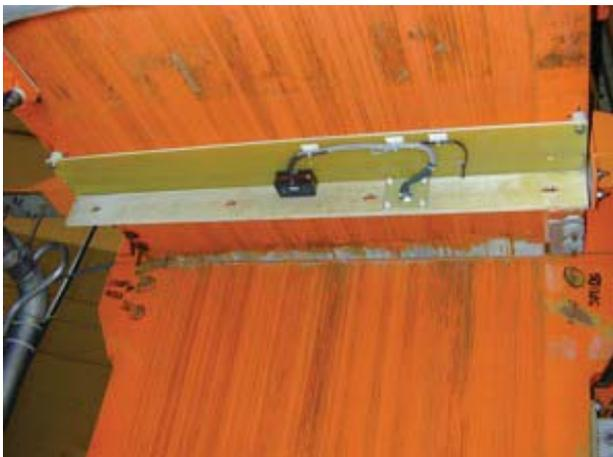
Figure 7: Outer probe as installed on limb 8-1, close to the outer vertical limb
