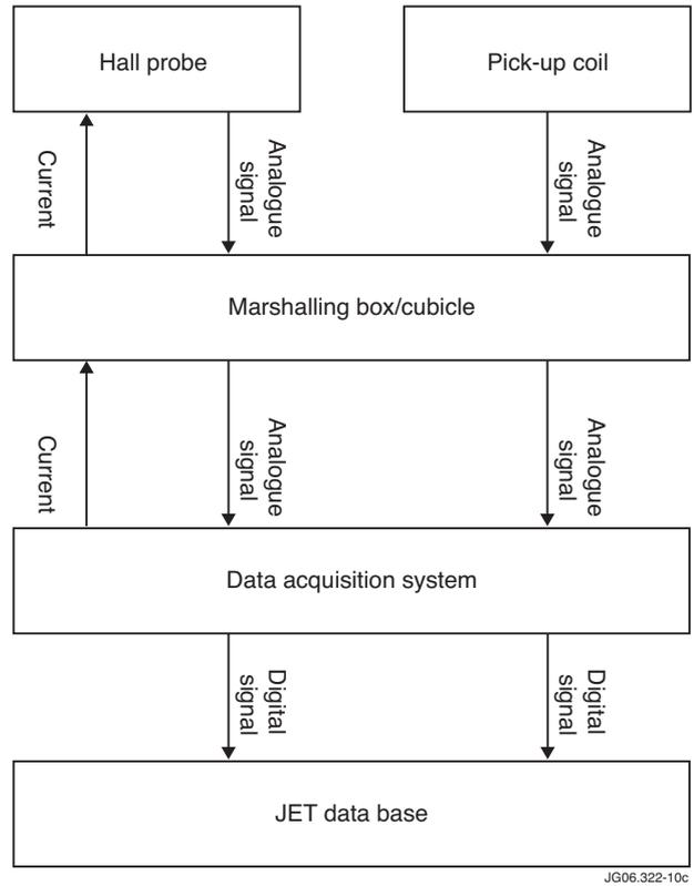
Figure 10: JET KC1E Data Acquisition System
