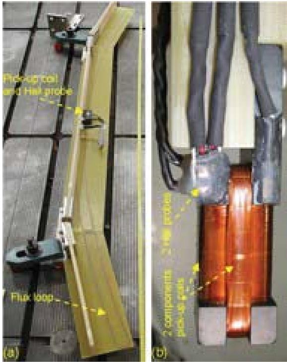
Figure 1: Limb probe subset for limb 3-4 (a); Collar probes (b)
