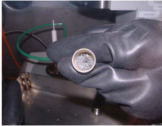
Figure 3: Picture of solid residue left after oxidation of the CFC flakes/dust
