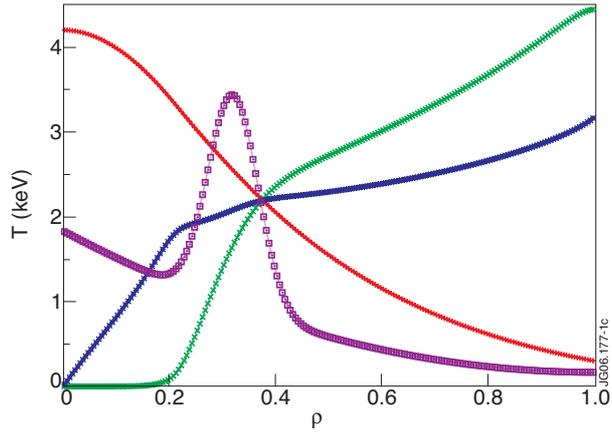
Figure 1: Profiles of temperature (red) (measured in keV), turbulence intensity (green),  $\kappa_T$  (blue) ( $\kappa_c = 1.8$ ) and source profile (magenta) ( $\rho = r/a$ ).
