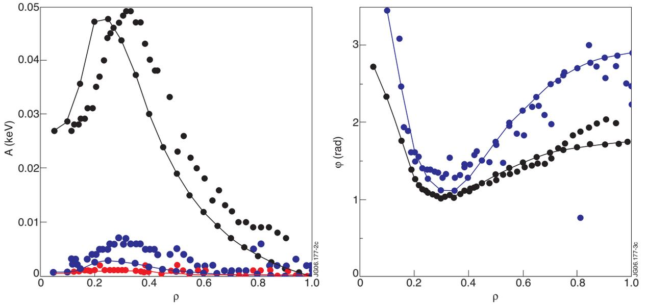
Figure 2: Fourier-analysis of the heat modulation in comparison with JET Pulse No: 55809, numerical results as lines points. Amplitude a) and phase b) evolution of fundamental (black), second harmonic (red) and third harmonic (blue).
