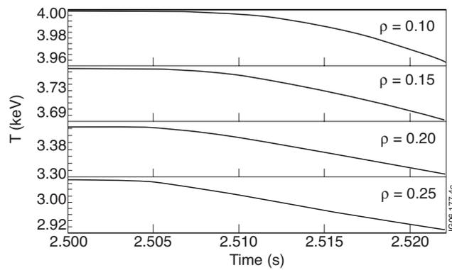
Figure 3: Evolution of the cold pulse.
