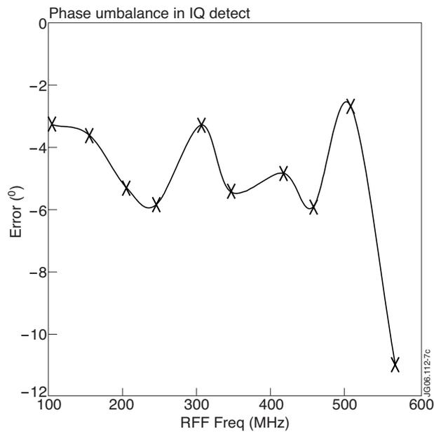
Figure 6: Quadrature detection phase error
