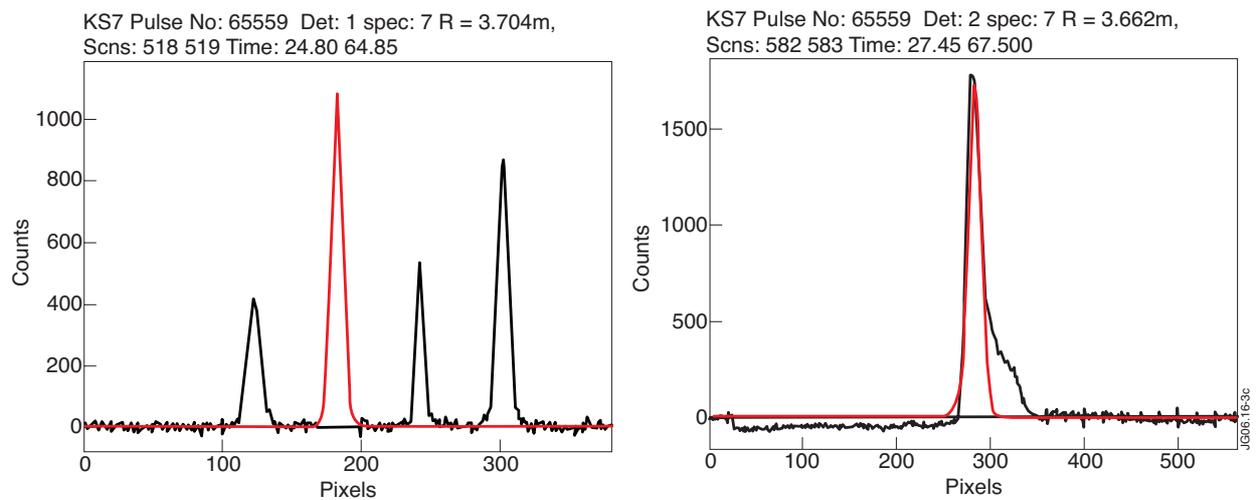
Figure 2: Example charge exchange spectra from C VI,  $n=8-7$  529.1nm for (a) Edge plasma view using McPherson 209, (b) Edge plasma using McPherson 205.
