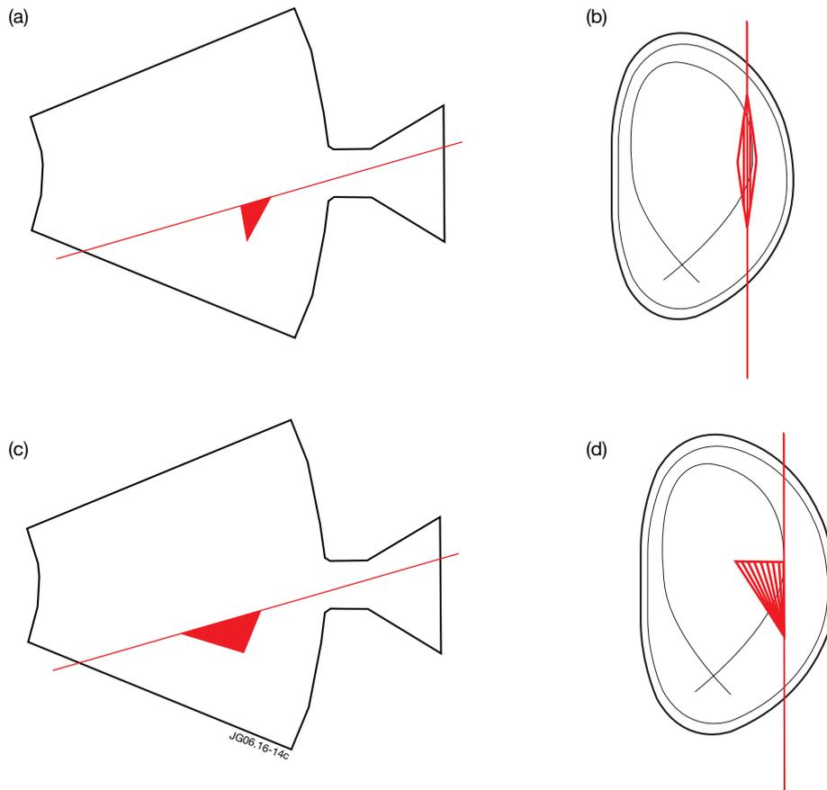
Figure 1: Layout of viewing lines of sight and neutral beams for JET's edge CXRS diagnostic. (a) Plan view of neutral beams and edge lines of sight and (b) Poloidal section. (c) Plan view of neutral beams and core lines of sight and (d) Poloidal section. The viewing lines of sight have both poloidal and toroidal components.
