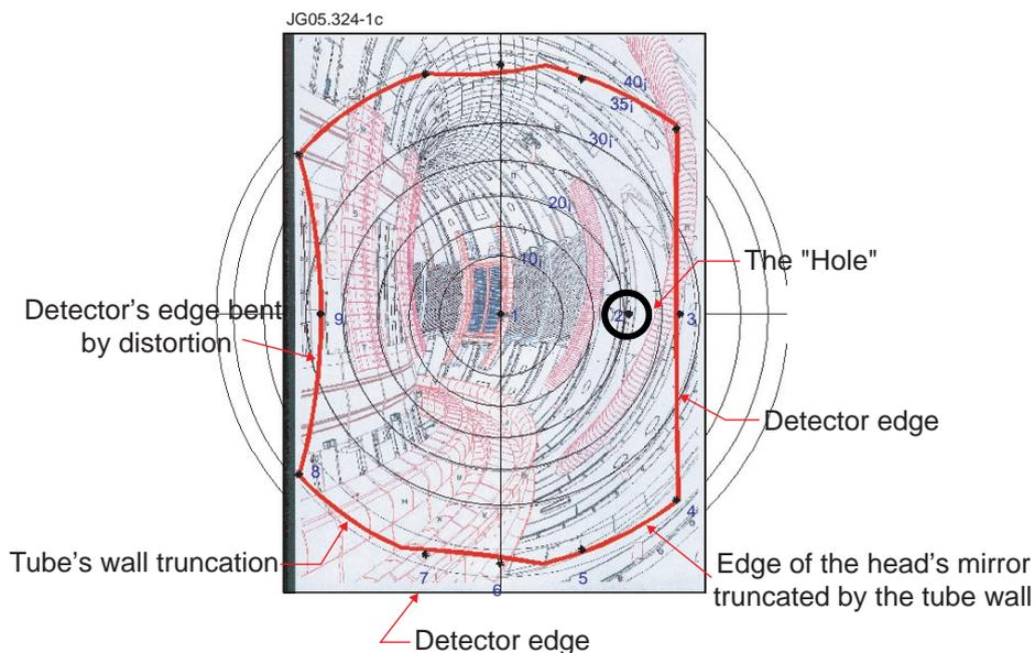
Figure 1: Field of view in the infrared and visible range
