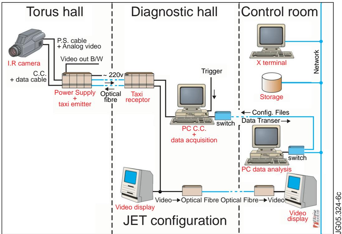
Figure 5: Schematic View of the data acquisition system
