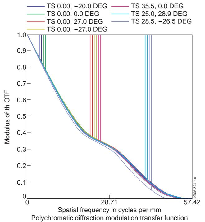
Figure 3: MTF curves of 9 points in the FOV
