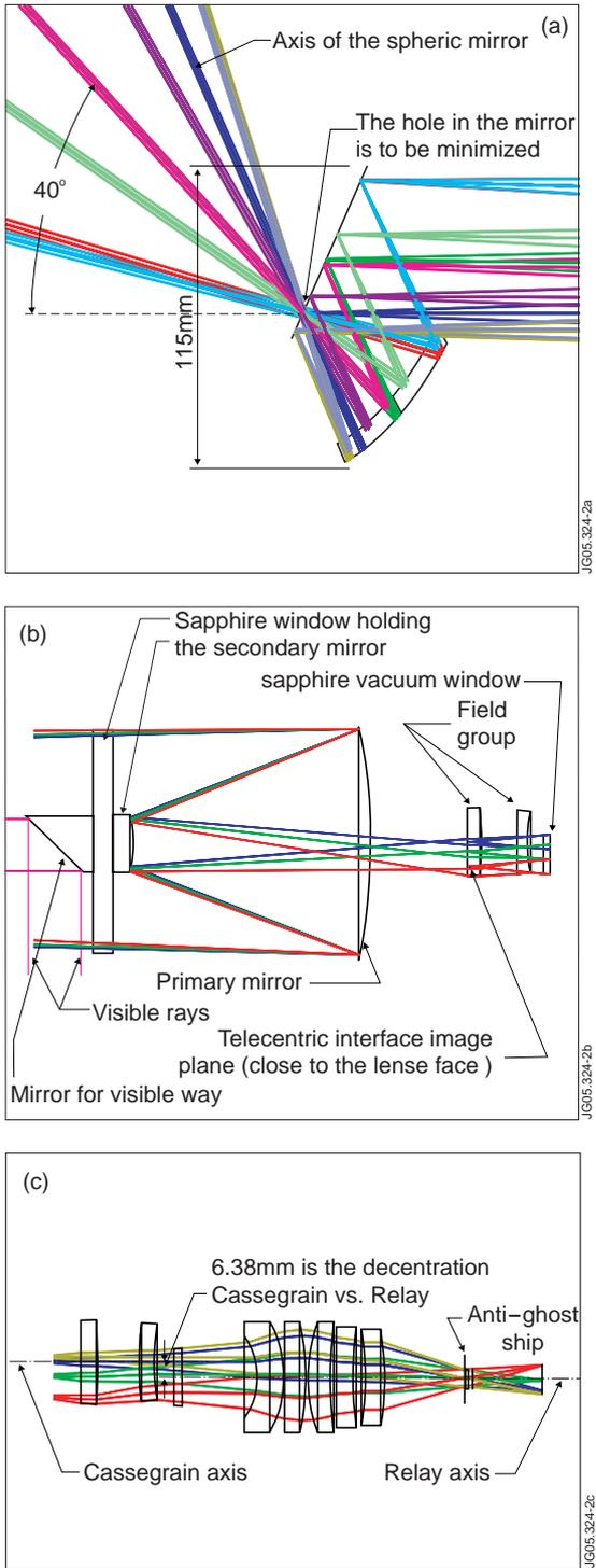
Figure 2: Optical design of the front mirrors (a), Cassegrain (b) and relay group lenses (c)
