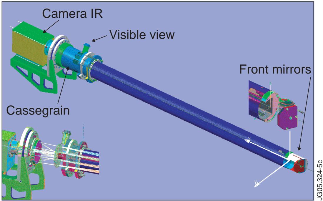
Figure 4: 3 D View of the opto-mechanical design
