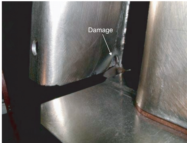
Figure 11: Bottom of flexipivot showing melted region.
