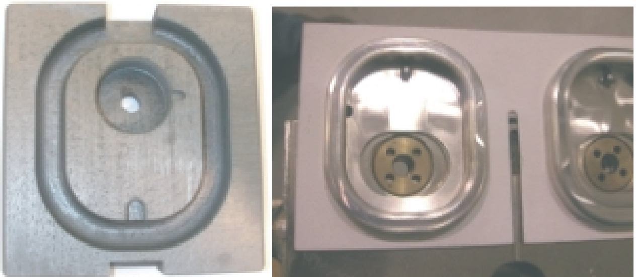
Figure. 4: One CFC tile with the groove for the Rogowski coil allocation. A detail of the halo sensor support structure where is visible the annular case that houses the Rogowski coil. The area outside the annular case has the alumina coating preventing the electrical contact of the tile with the structure.
