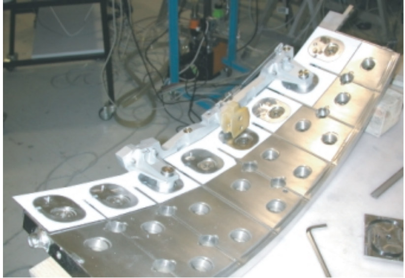
Figure. 5: The first halo sensor support structure installed on one spare protection plate. The support structure is attached to the remote handling tool that will be used for the installation.
