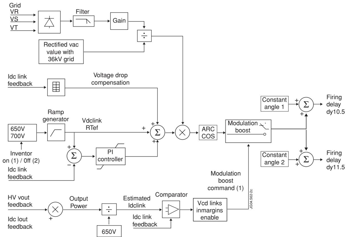
Figure 2: Control algorithm of the SCR Rectifier
