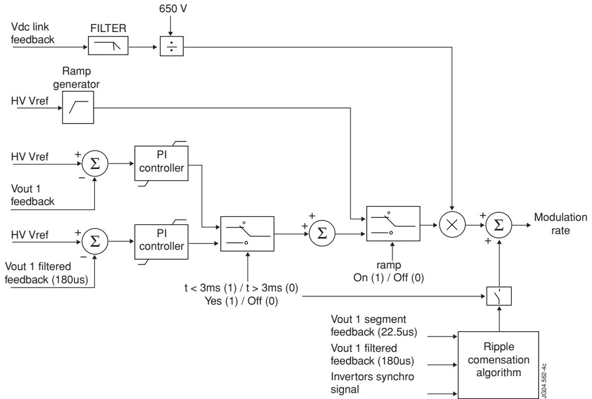
Figure 4: Control algorithm of the Invertor Control
