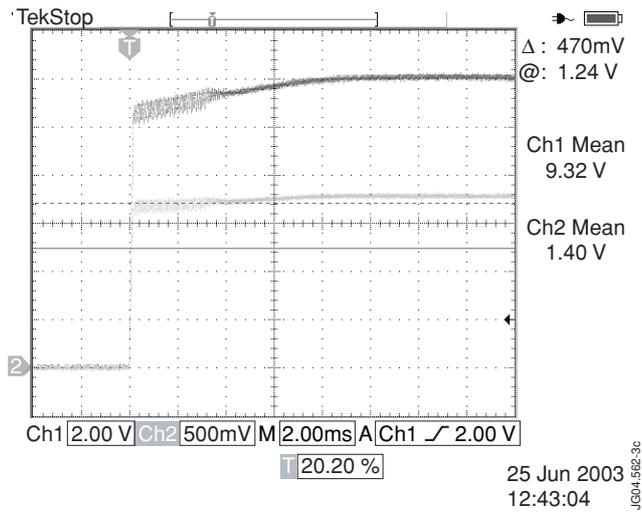
Figure 3: Ripple voltage reduction (CH1) after 3ms, at 120kV
