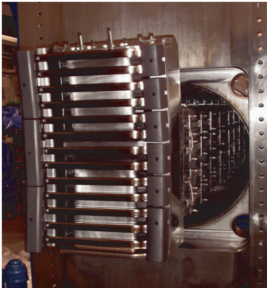
Figure 4: The High Power Prototype is full scale copy of the upper-left RDL of the JET-EP ITER-like Antenna.
