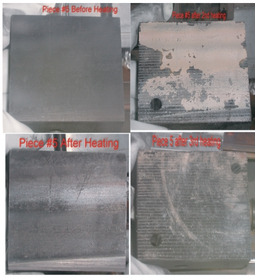
Figure 7: Photo of tile 7 after heating runs in test 4 (left top corner - before the heating, left bottom corner - after the first heating run, right top corner - after second heating run, right bottom corner - after third heating run)
