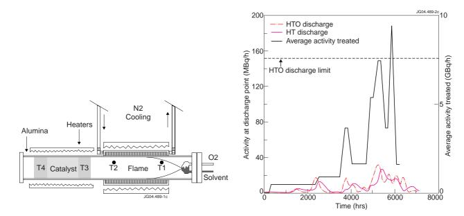
Figure 1: Cross-section of the furnace
