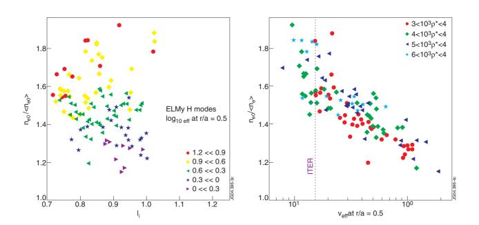
Figure 3: Peaking factor in H-mode versus  $v_{eff}$ . Symbols refer to classes if internal inductance.
