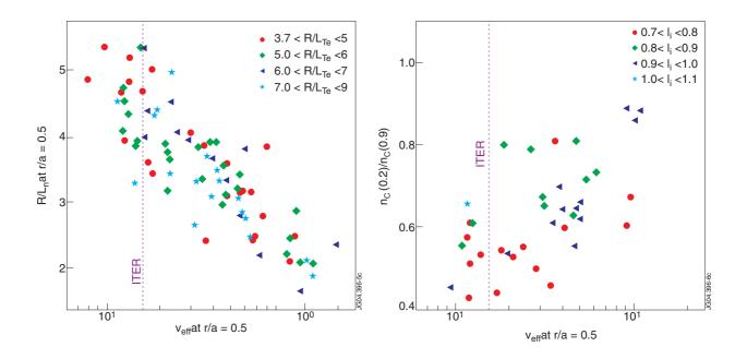
Figure 5: Normalised density gradient at r/a=0.5, resolved by temperature gradient (H-mode).
