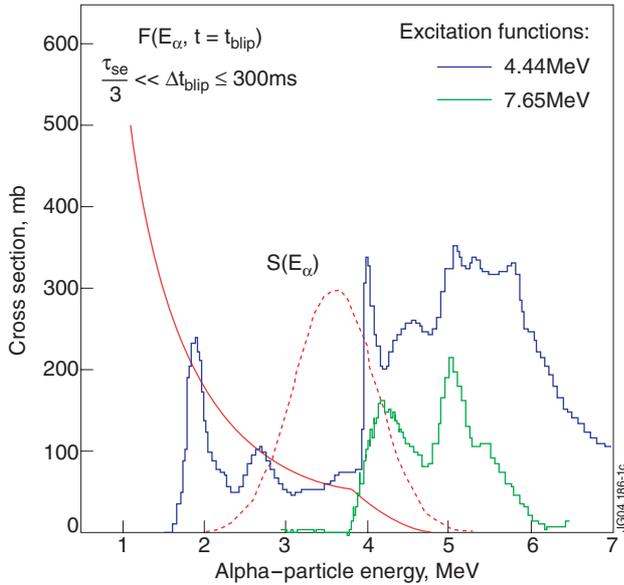
Figure 1: Excitation functions of  $^{12}\text{C}$  levels populated in the reaction  $^9\text{Be}(\alpha, n\gamma) ^{12}\text{C}$ . The  $\alpha$ -source distribution,  $S(E_\alpha)$ , was calculated for the 105keV T-beam injected in D-plasma;  $F(E_\alpha, t)$  - steady-state  $\alpha$ -particle energy distribution (a.u.).
