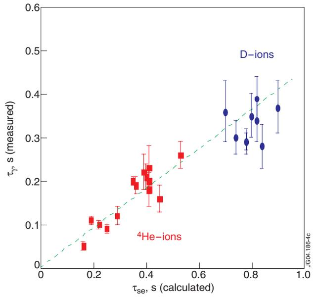
Figure 4: Measured 4.44MeV and 3.09MeV  $\gamma$ -ray decay-times for plasma scenario with:  $B_T=2.2\text{ T}$ ,  $I_p=2.2\text{ MA}$ .
