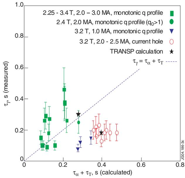
Figure 3: Measured 4.44MeV  $\gamma$ -ray decay-times for plasma scenarios with:  $B^T=2.25\text{--}3.2\text{ T}$ ,  $I_p=1.0\text{--}3.0\text{ MA}$ ;  $\tau_\alpha+\tau_T$  – classical slowing-down time of the fast  $\alpha$ 's and the beam tritons on electrons.
