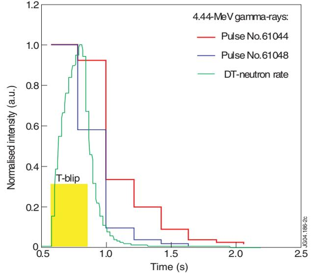
Figure 2: Comparison of evolutions of 4.44MeV  $\gamma$ -ray emission. Pulse No. 61044: 2.0MA/2.25T,  $P_{\text{DNBI}} \cong 14.5\text{MW}$ ,  $T_e(0) \cong 5\text{keV}$ . Pulse No. 61048: 2.0MA/2.25T,  $P_{\text{DNBI}} \cong 2.9\text{MW}$ ,  $T_e(0) \cong 3.5\text{keV}$ .
