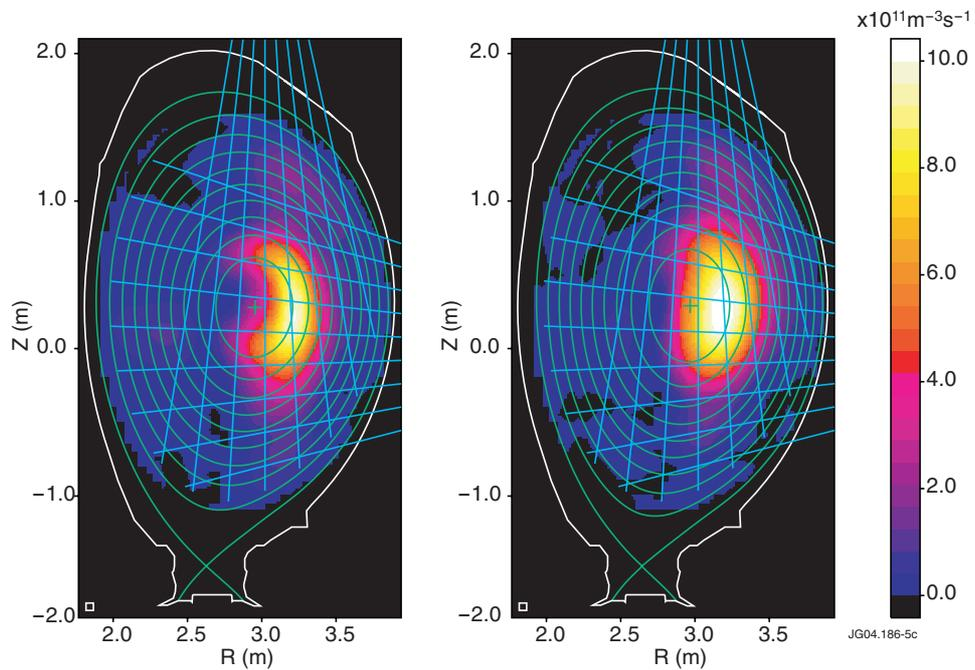
Figure 5: Gamma-ray images of a particles with  $E_\alpha > 1.7\text{ MeV}$  in 2.2T/2.0MA JET plasmas: left– with monotonic  $q$ -profile: right – with strongly reversed magnetic shear.
