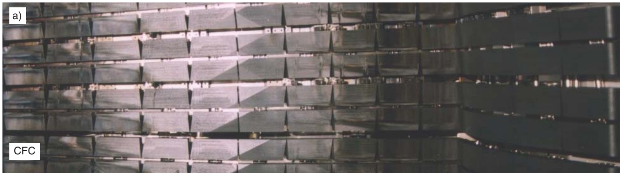
Figure 1: JET with the Mk-I beryllium divertor (a) and schematic view showing the location of tiles and Langmuir probes (b).
