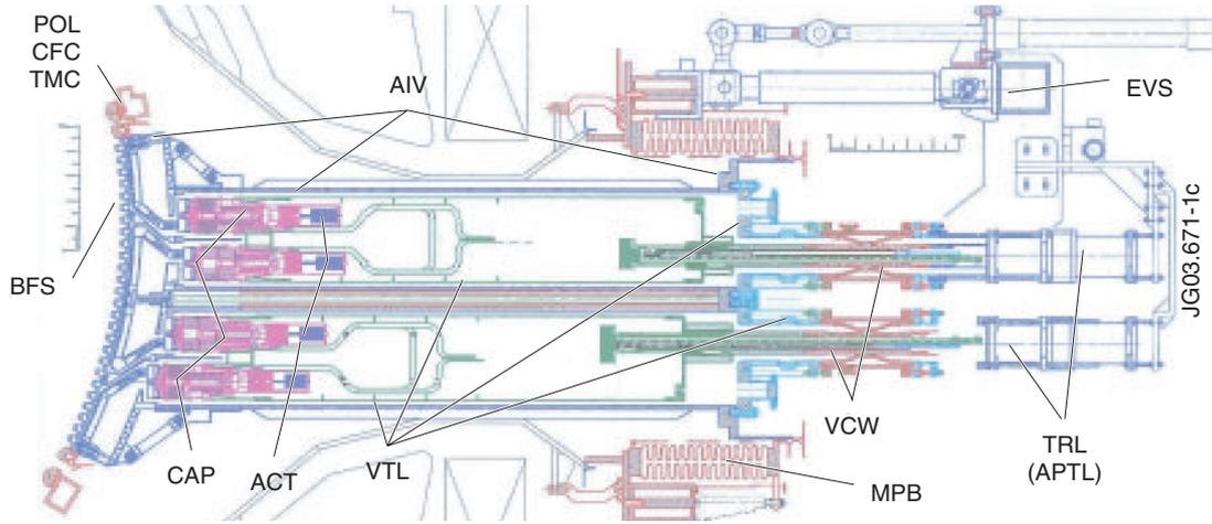
Figure 1: Cut view ITER-like ICRH Antenna showing the procurement packages (Table 1).
