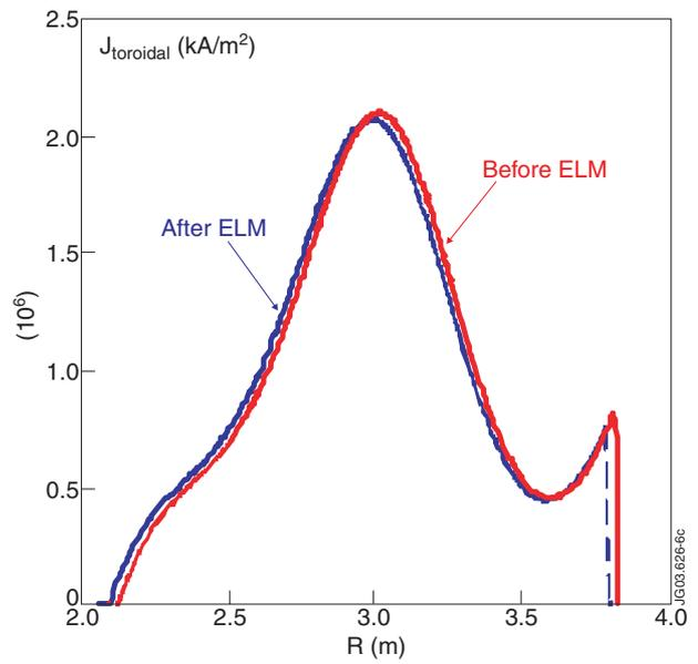
Figure 6: Toroidal current density as a function of major radius at axis height, (red) before ELM, (blue) after ELM
