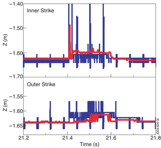
Figure 3: Strike jumps, inner and outer, measured with Langmuir Probes (blue) and position of maximum IR-measured temperature (red). Note: periodic (60ms) vertical jumps in LP meas. are an artefact to be ignored. JET Pulse No: 58837
