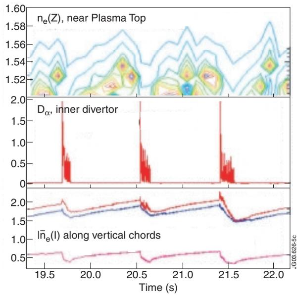
Figure 5: (a) Density profile (Li beam) (b):  $D_\alpha$  in inner divertor. (c):  $l \bar{n}_e$  along central inner (red), outer (blue) and edge (pink) vertical lines.
