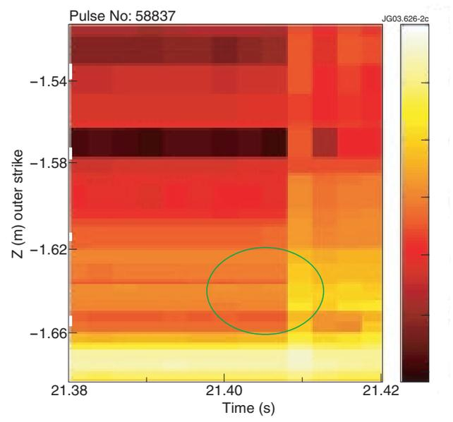
Figure 2: Outer strike jump, IR measurement.
