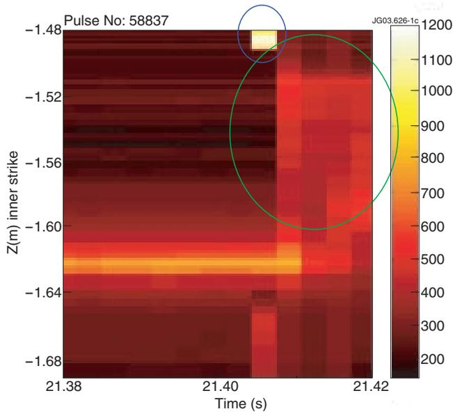
Figure 1: Inner strike jump, IR measurement.
