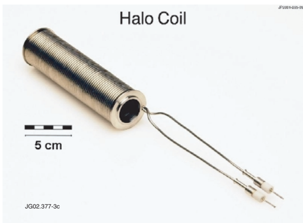
Figure 3: IUIWP toroidal field pick-up coil.
