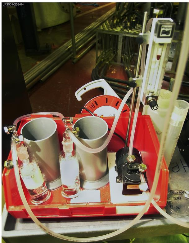
Figure 2: Shows a typical bubbler sampler system in operation in the torus hall. Two 250ml diffuser bottles (usually held within the grey plastic cylinders) are shown connected to the black pump unit via a manometer. The assembly is housed within a red plastic box to hold any possible spillage.
