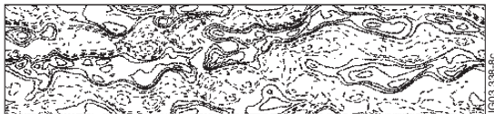
Figure 13: Characteristic \Delta contours of the ETG turbulence in the x - y plane [51].
