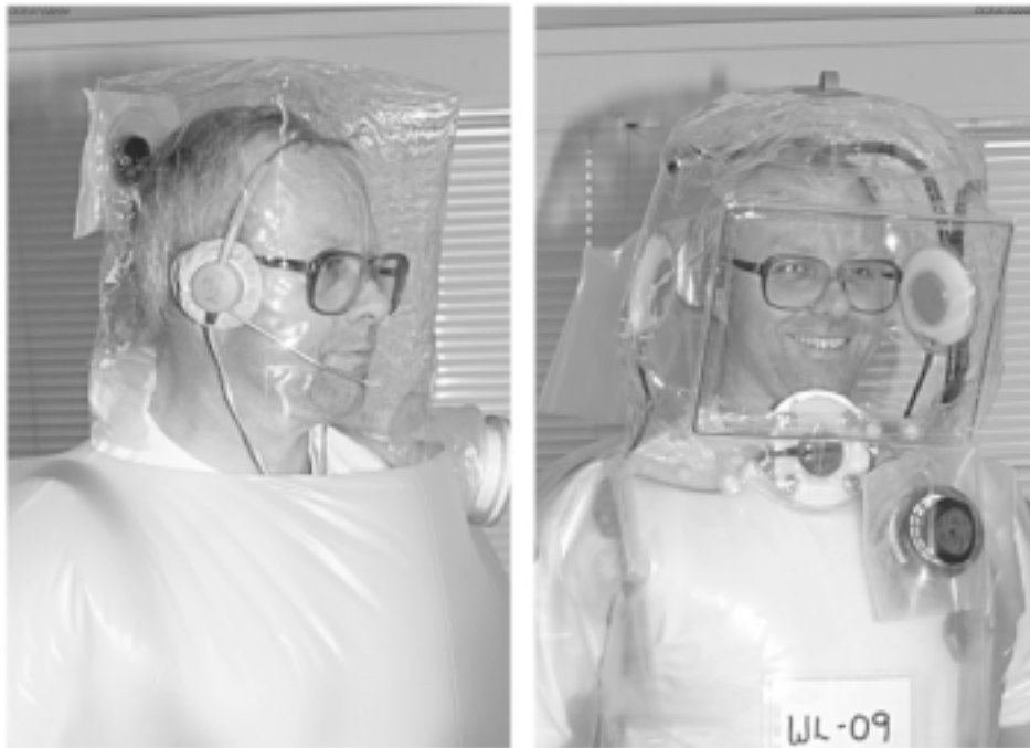
Fig.1: Binaural head sets within half suit (left). Speakers and a microphone in full suit (right).
